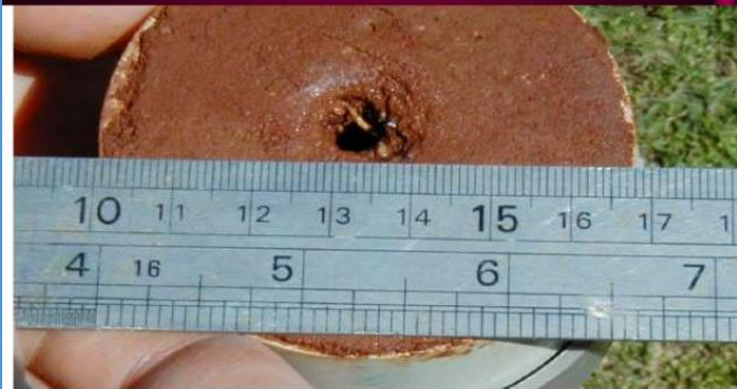
Pinhole test - completed pinhole size measurement
