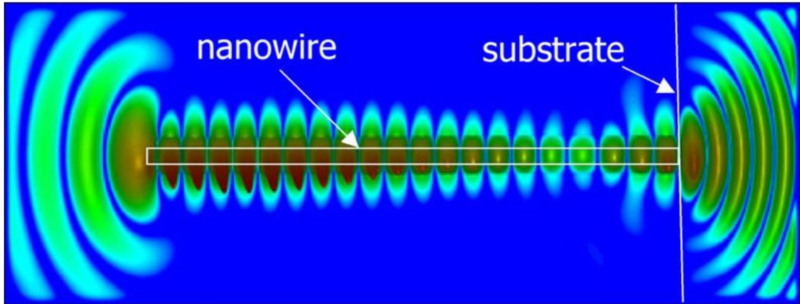
Light emission from a semiconductor nanowire - typically 10-100 nanometers wide and a few micrometers long-functions as a laser. Lasers made from arrays of these wires have many potential applications in communications and sensing
