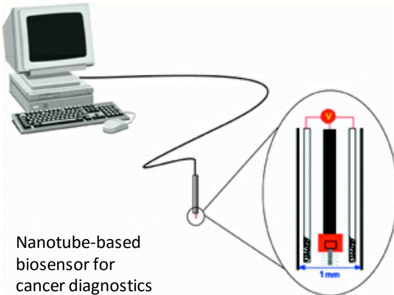
Nanotube-based biosensor for cancer diagnostics
