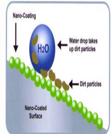
Glass is treated with chemical vapour method to deposit a mechanically stable nanolayer of titanium dioxide on the glass surface. (layer thickness ~50 nm)
