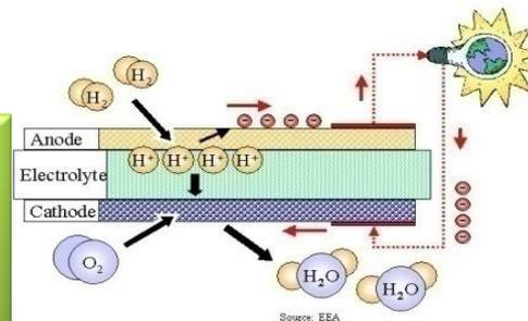
Schematic of a fuel cell
