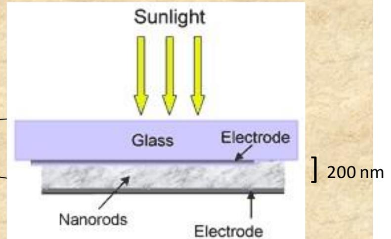
Nano solar cell: Inorganic nanorods embedded in semiconducting polymer, sandwiched between two electrodes
