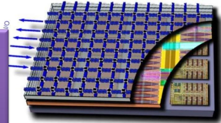
A silicon processor featuring on-chip nanophotonic network
